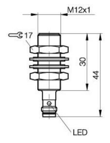
Inductive Sensors BES 516-325-G-E5-Y-S 49 M12x1 x 44 normally-open Sn=4mm shielded
